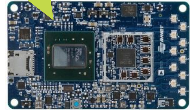
ADI AD9361 System on Module(SOM) SDR
